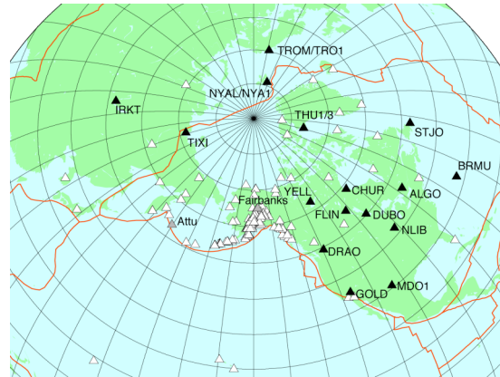
Fig. 1 Sites used in this study. White triangles show sites in the solutions used in the study, and black triangles are sites used to realize reference frame. No sites in Alaska are used to realize the reference frame because of earthquake displacements and non-linear postseismic motion, common problems in many regional networks. The gray triangles show the location of two test sites discussed in section 5.
